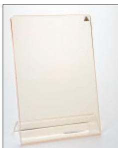
Beta and gamma radiation shields provide clear non-distorted vision, have comfortable angles for working on the bench top, and are easy to clean. We offer both sitting and standing versions. All shields are 27 x 20 x 15 cm.
